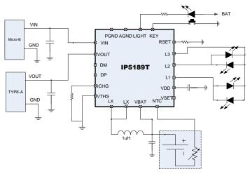
Fig1 Simplified application schematic (4 LEDs as the SOC indicator)
