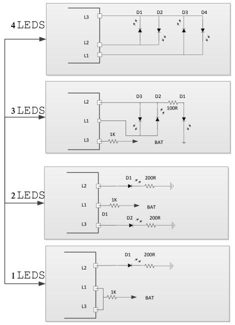
Fig 5 4/3/2/1 LED PIN configuration
