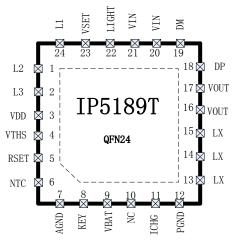
Fig 2 IP5189T Pin Diagram
