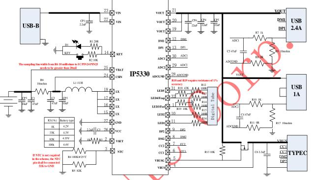
Figure 10 Typical Application Diagram (188 digital tube with OUT icon)
