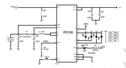
Fig 1 Simplified application schematic (4 LEDs as the SOC indicator)
