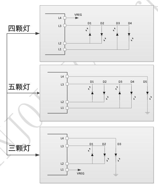
Fig 4 3/4/5 LED PIN configuration
