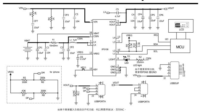
Fig 6 Typical application schematic with I2C
