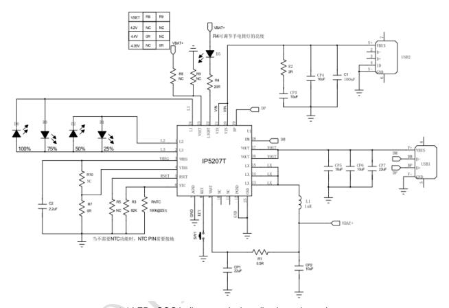
Fig6 4 LEDs SOC indicator typical application schematic
