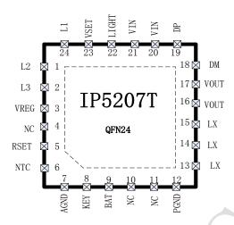
Fig 2 IP5207T Pin Diagram
