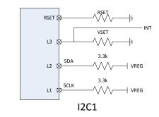
IP5322 support to connect with I2C1 or I2C2 at a time, when I2C circuit is deployed, the two pins will work as I2C\_SDA and I2C\_SCLK and the reused function will be disabled. Under I2C mode, INT signal is high-z at standby and high level at working state, which is used for waking up the MCU.
