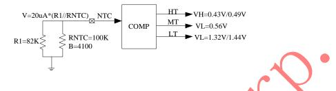
Figure 5 Battery NTC comparator
