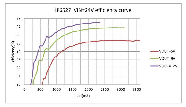
Figure 3. IP6527 output efficiency curve when VIN = 24V
