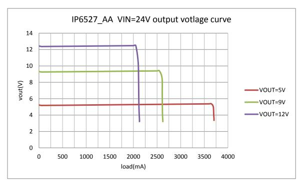
Figure 5. IP6527\_A Vout-lout curve when VIN=24V
