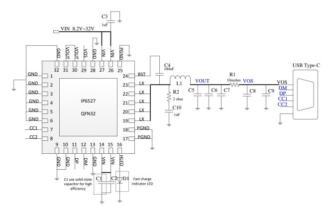
Figure 6. IP6527\_C Type-C output ports fast charge application schematic diagram
