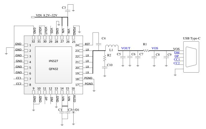
Figure 1. IP6527\_C simplified application schematic diagram
