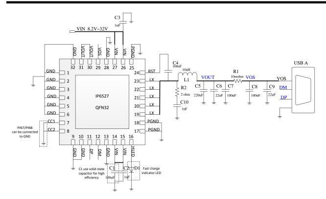
Figure 7. IP6527\_A USBA output ports fast charge application schematic diagram
