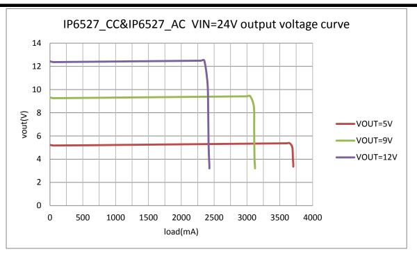
Figure 4. IP6527\_C Vout-Iout cureve when VIN=24V
