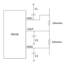
For IP6538 CC and IP6538 AC, different voltage is mapped to different current limit value shown below:
