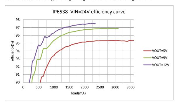
Figure 3. IP6538 output efficiency curve when VIN = 24V
