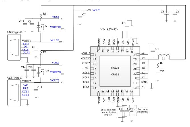
Figure 1. IP6538 CC dual USB Type-C output ports simplified application schematic diagram
