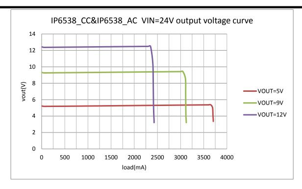
Figure 4. IP6538\_CC and IP6538\_AC Vout-lout cureve when VIN=24V
