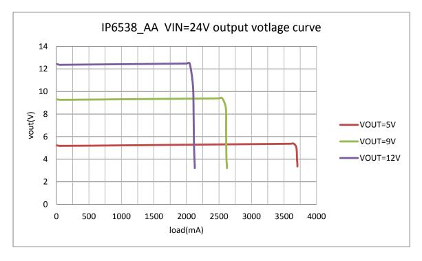
Figure 5. IP6538\_AA Vout-lout curve when VIN=24V
